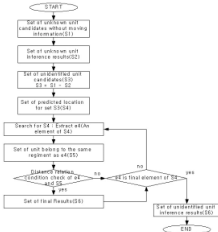
Figure 5.8: Flowchart of Rule execution for Unidentified Unit Inference
